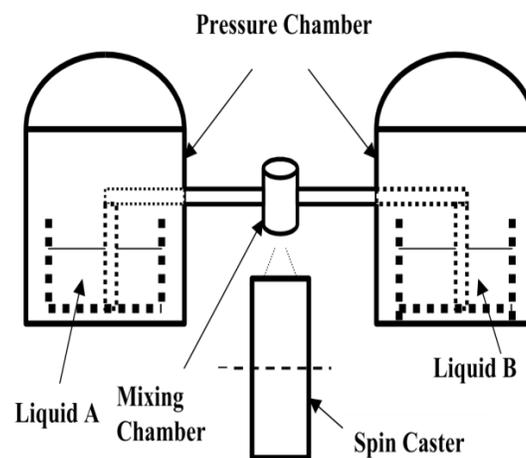
**Fig. 7. A Schematic Drawing of the Mixalloying Equipment. The metal was melted using induction heating. The equipment was about 15 feet high and occupied an area about 20' x 20', excluding auxiliary equipment such as power supply, water tank, metal chip collectors, etc.**
