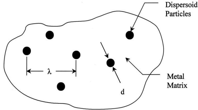
**Fig. 4. Microstructure of dispersion strengthened copper with hard ceramic particle.**
