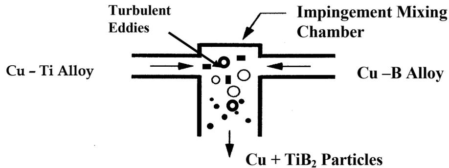
**Fig. 5. Mixalloy process for making dispersion-strengthened alloy. This figure shows impingement mixing of Cu/Ti liquid solution with Cu/B liquid solution to form a pure copper phase with nano-scale titanium diboride particles.**
