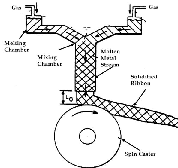
**Fig. 6. Spin casting that rapidly solidifies the molten copper/titanium diboride Liquid Stream from the mixalloy equipment.**
