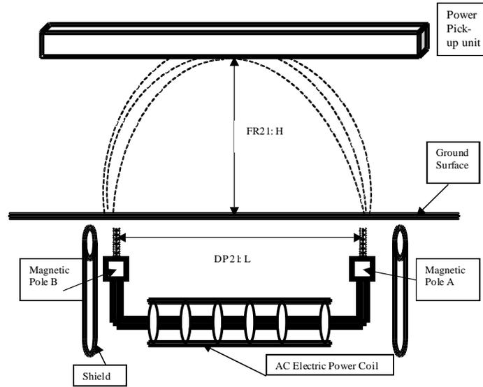
Fig. 1. Schematic drawing that shows the principle behind SMFIR.
