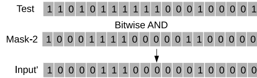
Fig. 6. Input' generation with bitwise AND of input bit sequence and Mask-2.
