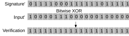
Fig. 7. Final bit sequence generated with bitwise XOR of Signature' and Input' bit sequences.
