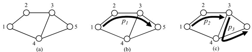
Fig. 1. (a) A network with 5 nodes. (b) Single-hop routing. (c) Multi-hop routing.
