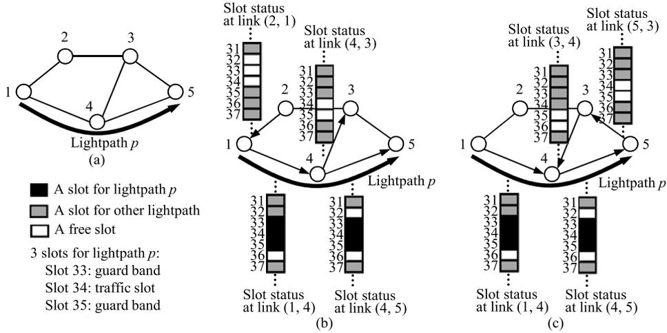
Fig. 3. (a) A lightpath  $p$  in a network with 5 nodes. (b) Misalignments created due to the allocation of slots 33, 34, and 35 to lightpath  $p$  at link (1, 4). (c) Misalignments created due to the allocation of slots 33, 34, and 35 to lightpath  $p$  at link (4, 5).
