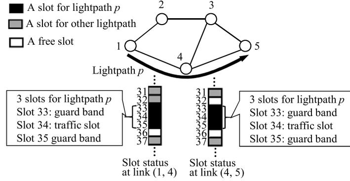
Fig. 2. A lightpath  $p$  in a network with 5 nodes.
