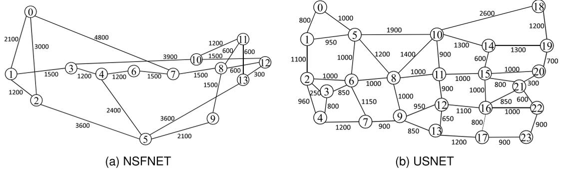
Fig. 6. (a) The topology of the 14-node NSFNET with 21 bidirectional links. (b) The topology of the 24-node USNET with 43 bidirectional links.
