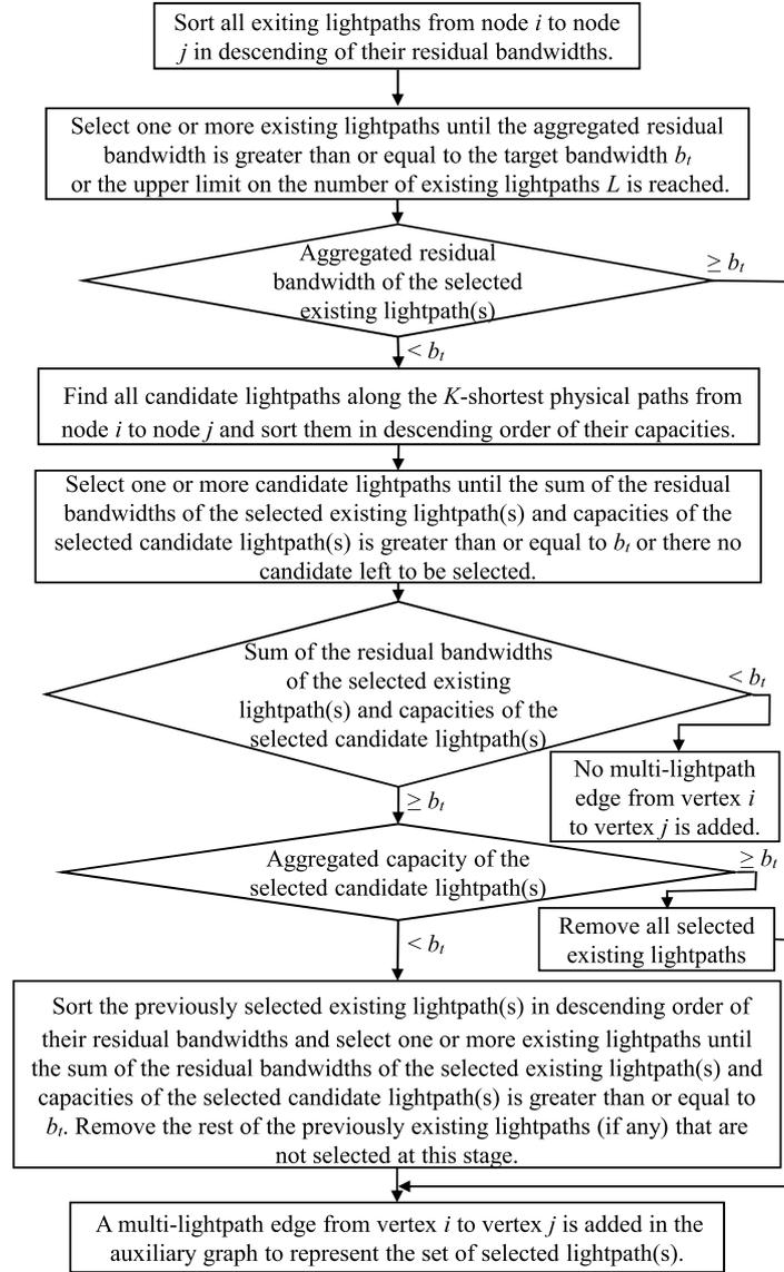
Fig. 5. The flowchart for trying to add a multi-lightpath edge from vertex  $i$  to vertex  $j$  in the auxiliary graph.
