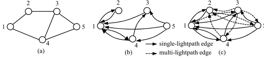
Fig. 4. (a) A network with 5 nodes. (b) Auxiliary graph with only single-lightpath edges. (c) Auxiliary graph with single-lightpath and multi-lightpath edges.
