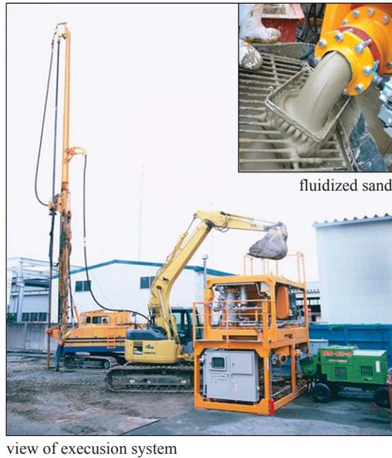
Fig. 1. SAVE-SP machine and mixing plant.
