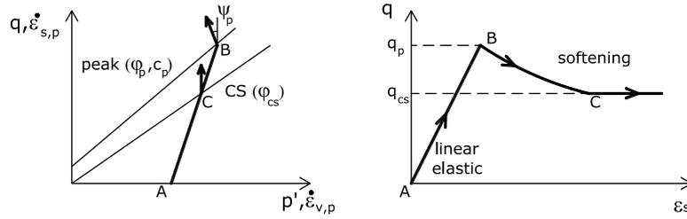
Fig. 4. SS response for conventional drained triaxial compression test.
