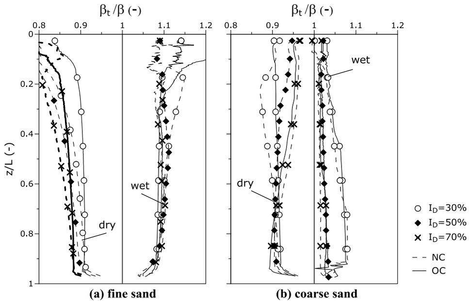
Fig. 14. Load tests - results of the analyses for long piles ( $L=40$  m):  $\beta_t/\beta$  for (a) fine and (b) coarse sands.
