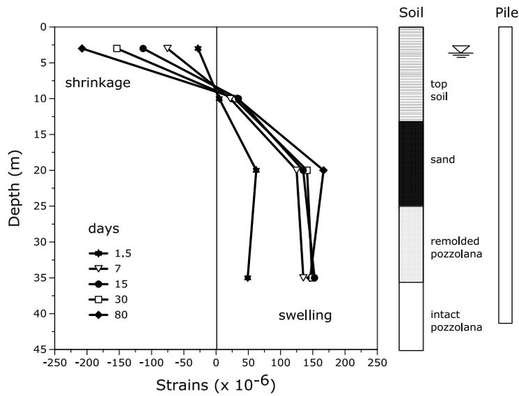
Fig. 1. Measured strains after casting (data from [12]).
