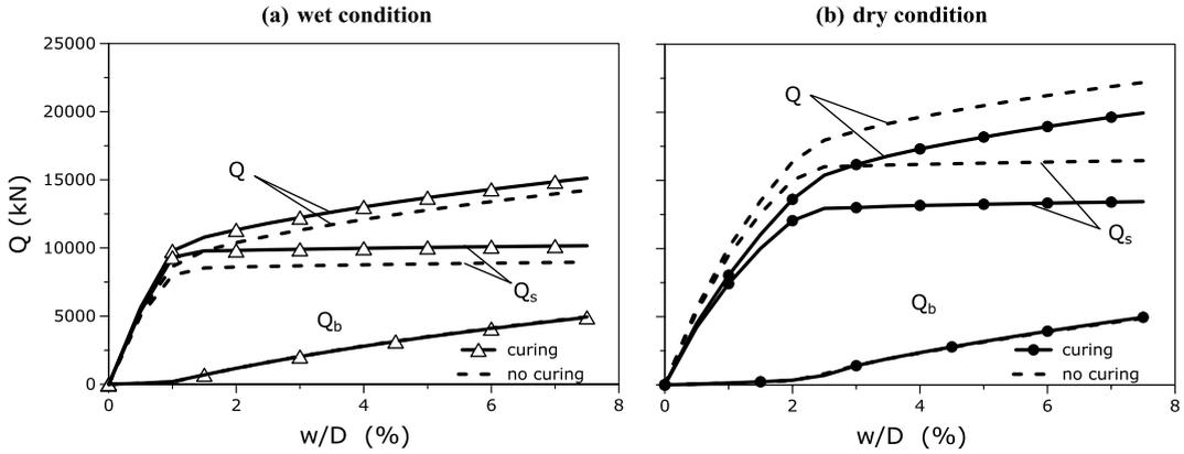
Fig. 10. Single pile: load-displacement curves in (a) wet and (b) dry conditions, with and without concrete curing simulation.
