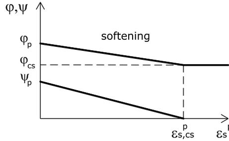
Fig. 5. Linear reduction for angle of friction and dilation.
