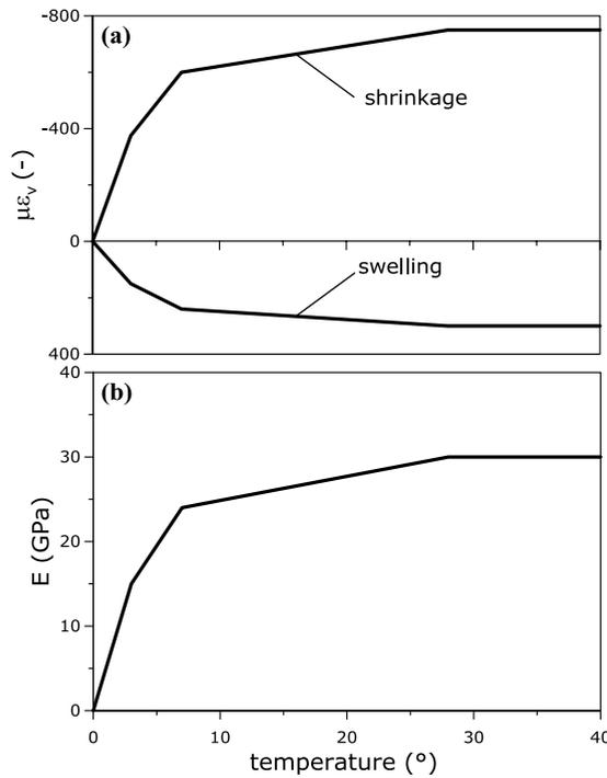
Fig. 7. Concrete curing: (a) volumetric strains and (b) stiffness evolution.
