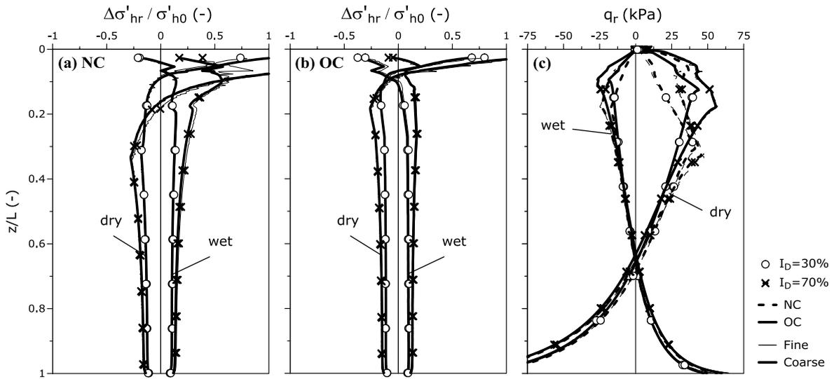
Fig. 13. Concrete curing - results of the analyses for long piles ( $L = 40$  m): horizontal stress changes in (a) NC and (b) OC soil; (c) residual shear stresses.
