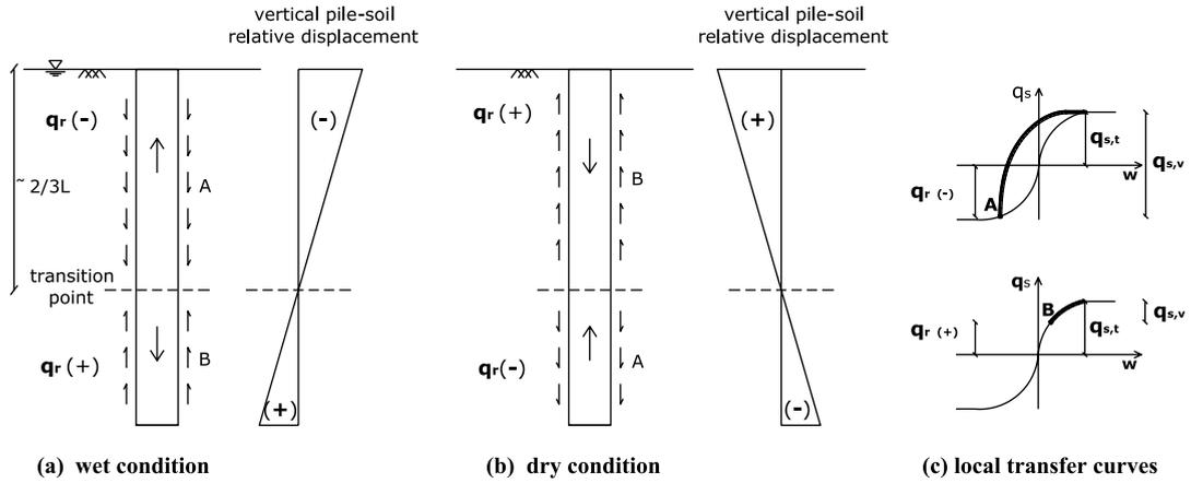
Fig. 3. Effects of concrete curing on a floating pile in (a) wet and (b) dry conditions; (c) “true” and “virtual” values of shaft friction on local transfer curves.
