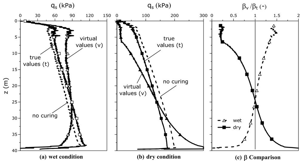
Fig. 11. Single pile: “true” and “virtual” shear stress profiles in (a) wet and (b) dry conditions, with and without concrete curing simulation; (c) comparison between “true” and “virtual”  $\beta$  values.
