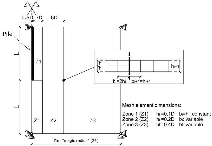
Fig. 6. Finite different mesh adopted for the analyses.
