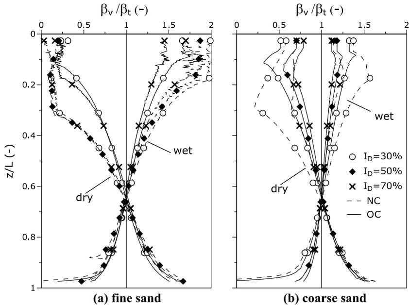
Fig. 15. Load tests - results of the analyses for long piles ( $L=40$  m):  $\beta_v/\beta_t$  for (a) fine and (b) coarse sands.
