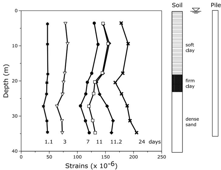
Fig. 2. Measured strains after casting (reproduced from [13]).
