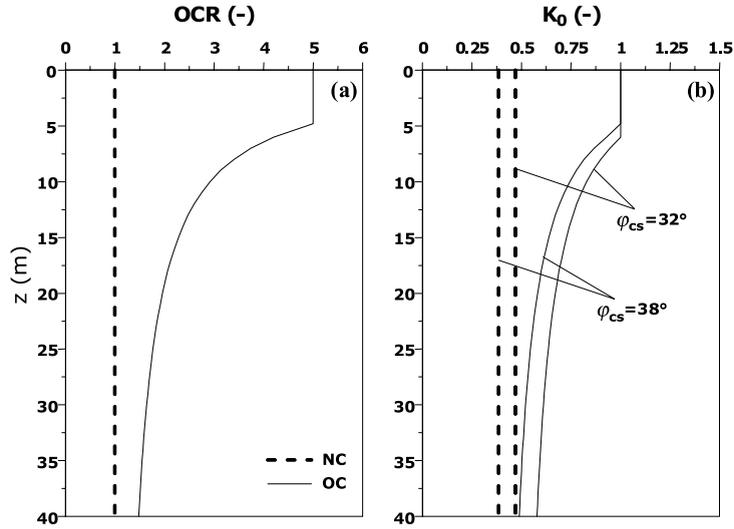
Fig. 12. Parametric analyses: (a) OCR and (b)  $K_0$  profiles for NC and OC models, changing  $\varphi_{cs}$ .
