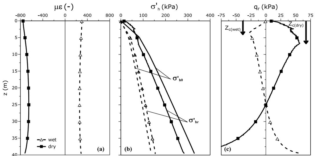
Fig. 9. Concrete curing of a single pile: (a) pile deformations, (b) horizontal and (c) shear stresses.
