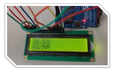
Fig. 4. Temperature sensor and Arduino board.
