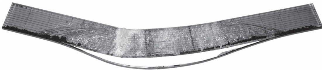
Fig. 15. Typical distributed cracking in ADH-PT specimens and significant yielding of tendon.
