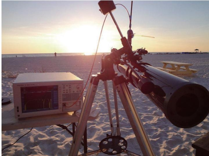
Fig. 6. View of the experimental set up used for the measurement of the IRS of the entire visible spectrum of Sunlight showing the telescope and the Yokogawa analyzer AQ6373 set for the detection at the horizon.
