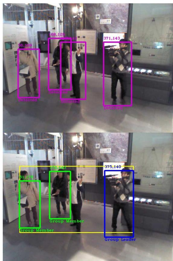
Fig. 14. Video 3 with 46% of accuracy. Top: All individuals have been detected, no roles assigned yet. Bottom: The cameraman has been addressed as the group leader, whereas the science communicator is not even detected on this frame. A large motion rectangle is displayed containing all the detections on scene.
