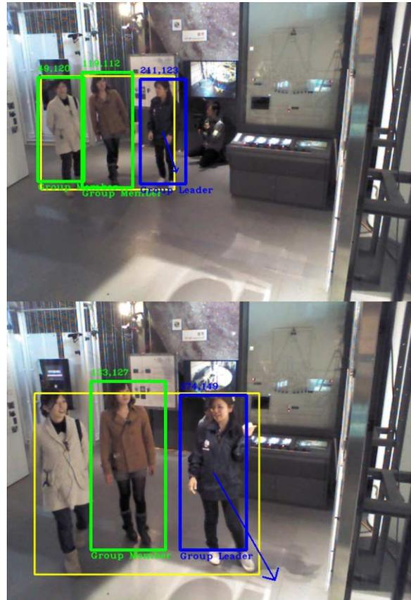
Fig. 10. Video 5 with 98% of accuracy. Top: Sample frame 5. A blue arrow with the leader's torso as origin estimates her direction. Bottom: Sample frame 15. Leader's direction arrow indicates the direction of movement and also displays its proportional magnitude.
