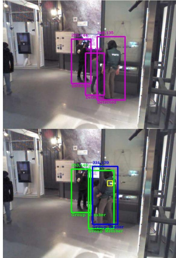
Fig. 6. *Training3* video exemplifying a Soft case. Top: Frame 1, the people detector outputs three human detections on scene. Bottom: Frame 35, the algorithm is able to rapidly categorize all the detections after the group leader has been identified.
