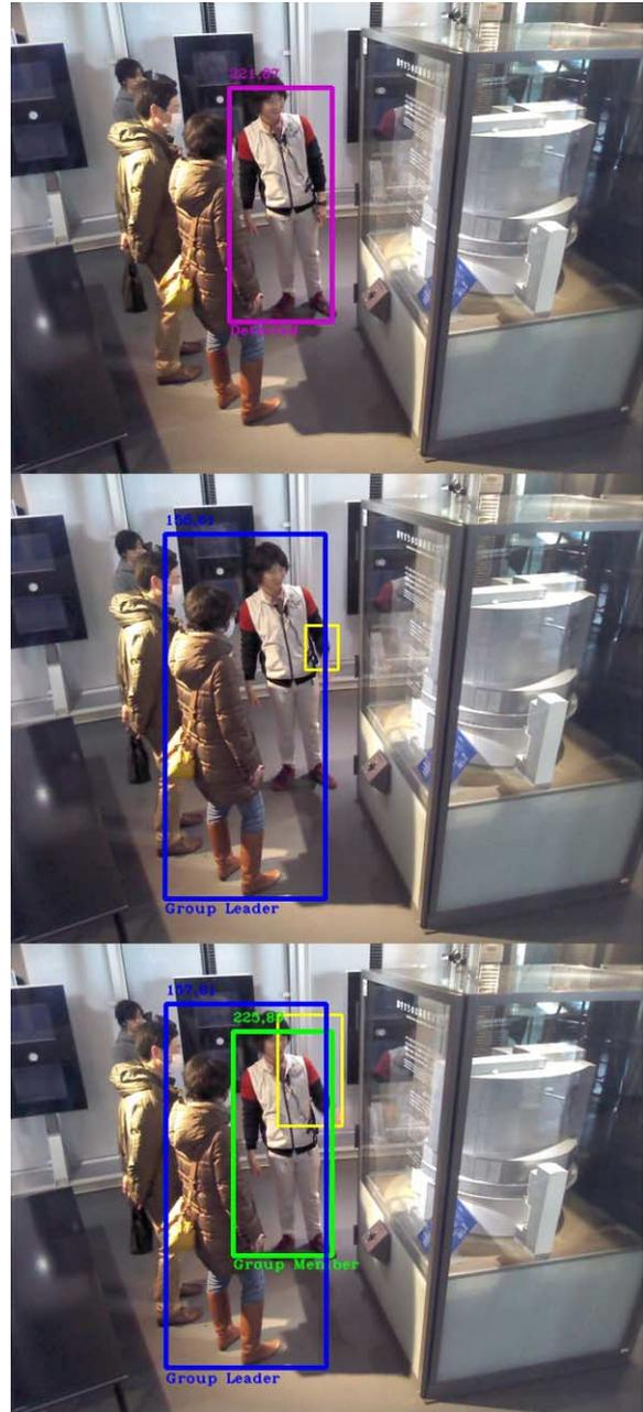
Fig. 12. Video 1 with 36% of accuracy. Top: Frame 1, science communicator has been detected, no role assigned yet. Middle: Frame 4, science communicator gestures and motion box overlaps with the only detection obtained, selecting a museum visitor as the group leader. Bottom: Frame 6, science communicator is detected after the leader role has been given, appointing him as a group member.
