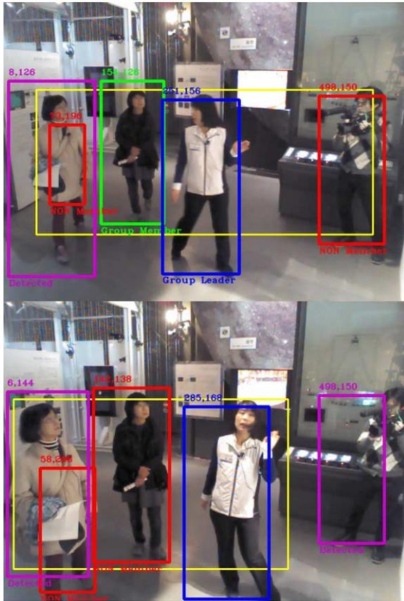
Fig. 17. Video 3 results under exponential motion implementation. Top: Frame 51, although the four people on the scene are moving as significantly as the group leader does, the leader is correctly categorized along with the cameraman and one of the two group members. Bottom: Frame 102, two out of three detections are wrongly categorized. Purple boxes are references to previous detections.
