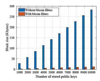
Fig. 12. Status ledger's block size with and without using BF. [11].
