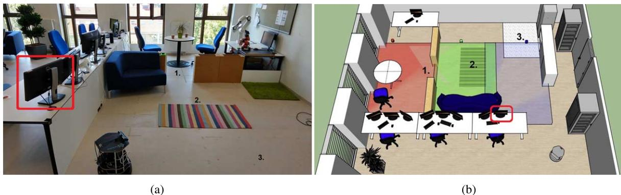
Fig. 4. Image and 3D sketch of the lab environment. The three evaluation scenarios are numbered, and the three cameras' fields of view are visualized in red, green and blue. The position of the smart display for feedback is encircled in red, and the mobile robot's initial pose is depicted in the bottom right of the sketch.
