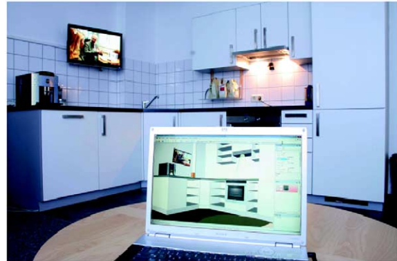
Fig. 6. The programme on the TV set is reflected in the virtual model (laptop in the foreground). A context menu in the model acts as a remote control to switch channels; also the hood light is in sync between both realities.
