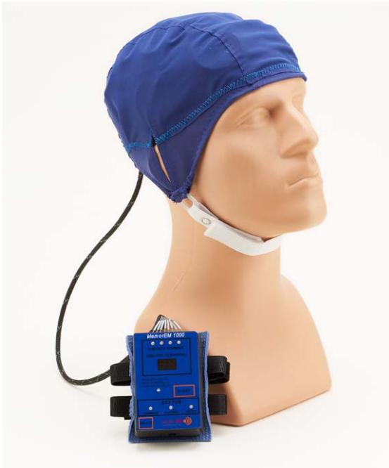
Fig. 3. A MemorEM device being worn by a mannequin human head. The control panel/battery box is worn on the subject's upper arm and is wired via a cable to eight radiofrequency wave emitters (four on each side of the head) embedded between the device's two-layered head cap. Emitters collectively provide full forebrain TRFT, while allowing near complete mobility during any given 1-hour treatment.
