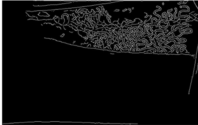
Fig. 8. Waterline detection: result after applying the Canny edge detection. The random pattern drawn on the hull to improve the disparity map is only detected above water level. The waterline itself is clearly distinguished. The edges detected on the side of the frame and at the bottom of the image are removed using a mask.
