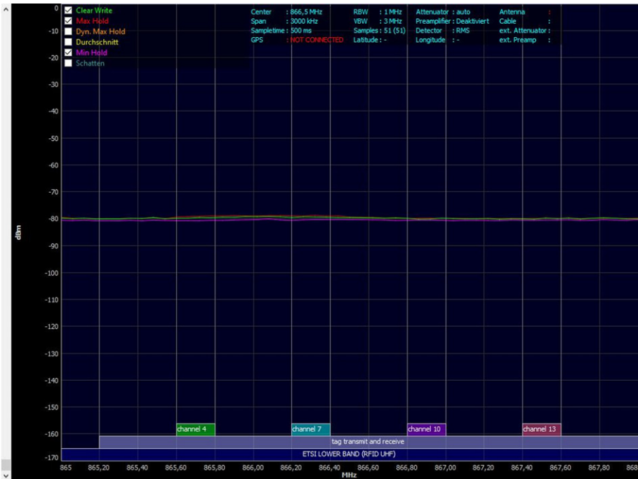
Fig. 7. Measurement of the power in the UHF RFID frequency range at the RFID testcenter.
