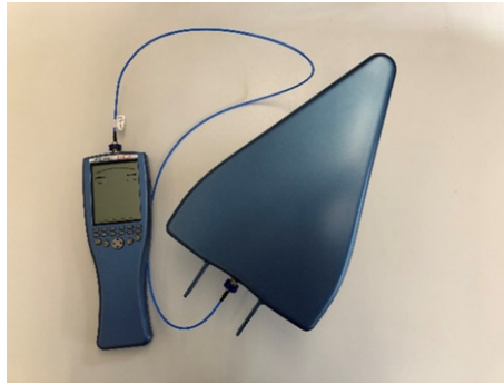
Fig. 4. Aaronia SPECTRAN HF-60100 handheld spectrum analyser with UHF antenna.
