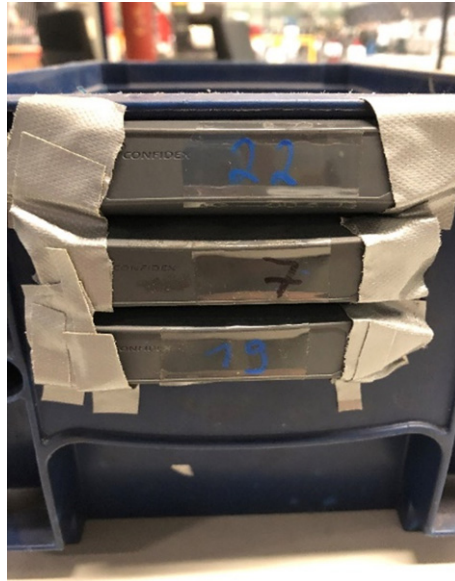
Fig. 20. Attachment of the RFID tags to the load carrier with a distance of 0 cm.
