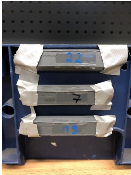
Fig. 21. Attachment of the RFID tags to the load carrier with a distance of 1 cm.
