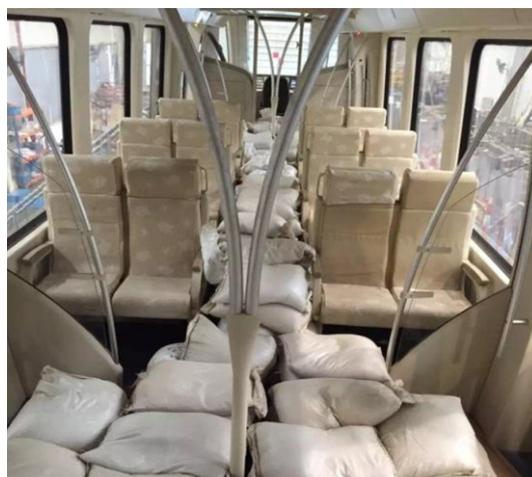
Fig. 18. The photograph of load-carrying test in vehicles operating on Changsha Maglev Express Line.
