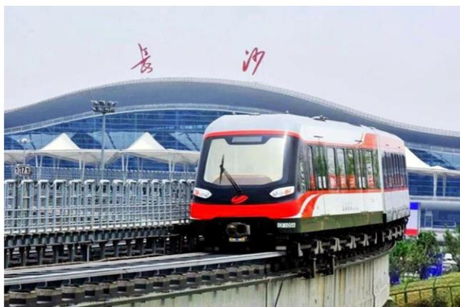
Fig. 1. The photograph of medium-low speed maglev train in Changsha.
