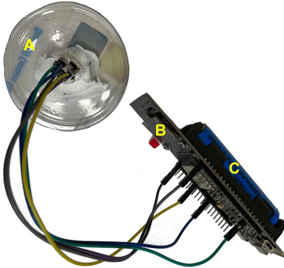
Fig. 3. Low-cost prototype for monitoring and estimating the HR and its main component: (A) INMP441 MEMS microphone, (B) ESP32-based microcontroller and (C) power battery.
