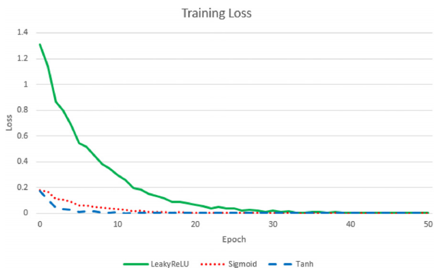
Fig. 1. Training Loss of three different activation functions.
