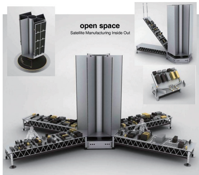
Fig. 9. Communication satellite open space architecture to tackle the common (75%) late box replacement issue. Note the flower inspired panel setup around a core structure. Heat pipes regulate temperature ( ME310 EXPE 2011 , 2011).
