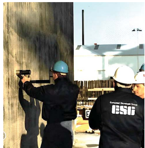
Fig. 23. Steel slipform used for the caissons (left), and CAPO-Testing (right).
