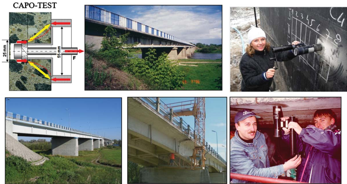
Fig. 34. Examples of Polish bridges tested for upgrading –higher loading– shown with CAPO-TEST.
