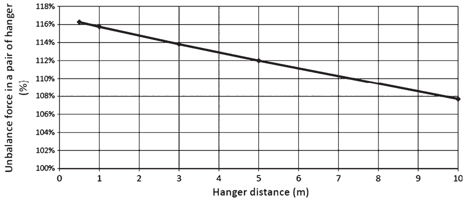
Fig. 6. Unbalanced forces in a pair of hangers.
