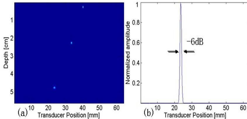
Fig. 4. The synthetic aperture image reconstruction in the simulation and the spatial resolution of the third point target at a depth of 48 mm.
