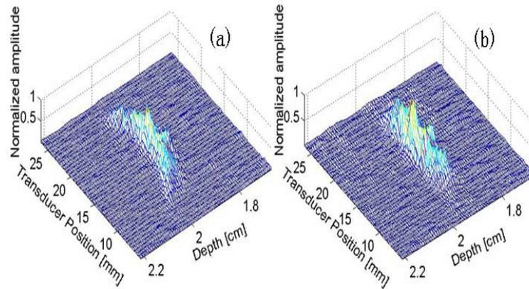
Fig. 6. The recorded one-point hologram data and the geometric distortion compensation result. The one-point in the red rectangle at a depth of 19mm is selected in Figure 7(a). The curve hologram data is converted into linear data, which demonstrates that the geometric distortion compensation is achieved.
