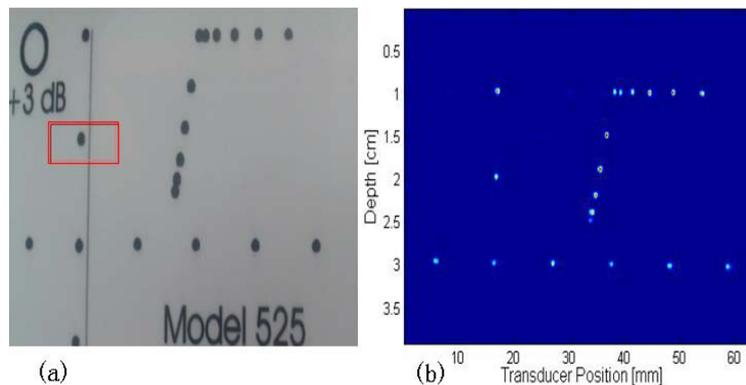
Fig. 7. The part screen capture of phantom and the corresponding synthetic aperture ultrasonic holographic imaging after the geometric distortion compensation.
