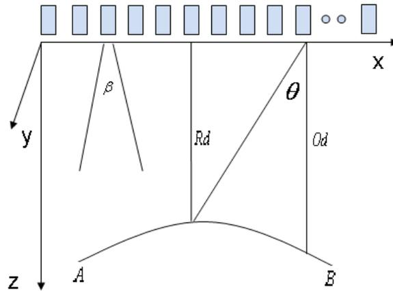
Fig. 1. Geometric distortion in the imaging x-z-plane. The individual transducer element conducts a fairly wide-angle  $\beta$  beam in the plane of imaging.
