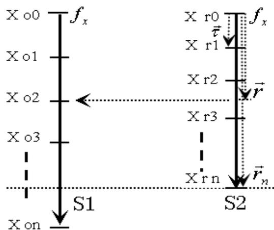
Fig. 2. A spatial frequency component is given as an example so as to illustrate the operation of spatial compression and re-sampling in the frequency domain.
