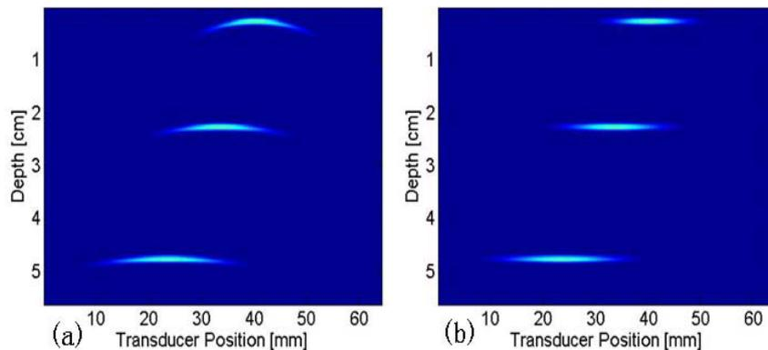
Fig. 3. Geometric distortion in the simulation hologram data without compensation is shown in (a). The compensation result is shown in (b).
