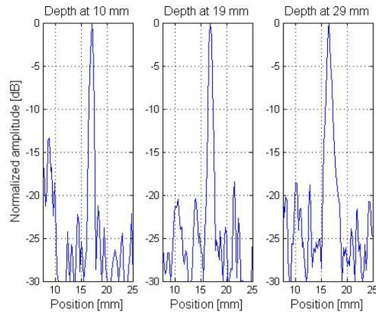
Fig. 8. The -6dB spatial resolution is about 1 mm and is approximately uniform throughout the depth range. Three point scatters in Figure 7(b) at transducer position 16mm and depth 10 mm, 19 mm, 29 mm are selected respectively and their corresponding intensity curves for the lateral direction are also shown.
