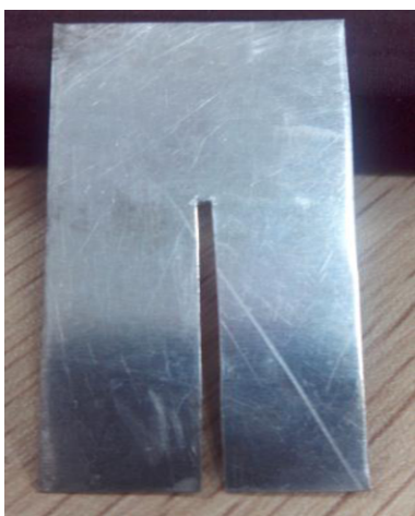
Fig. 8. The phantom of a strong reflection surface with a stripped opening of 1.5 mm width.
