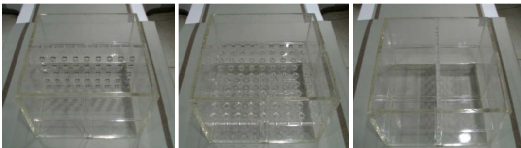
Fig. 2. Multi-orientated water-phantom in (a) axial (b) coronal and (c) sagittal configurations.
