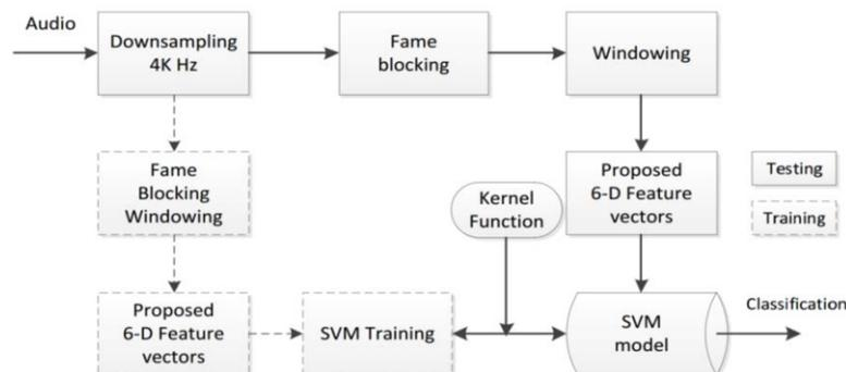
Fig. 1. Block diagram of the snoring classification system.
