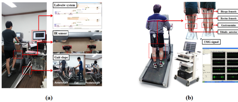
Fig. 2. (a) Experiment picture for measurement of IR sensors, (b) Experiment picture for measurement of electromyography.
