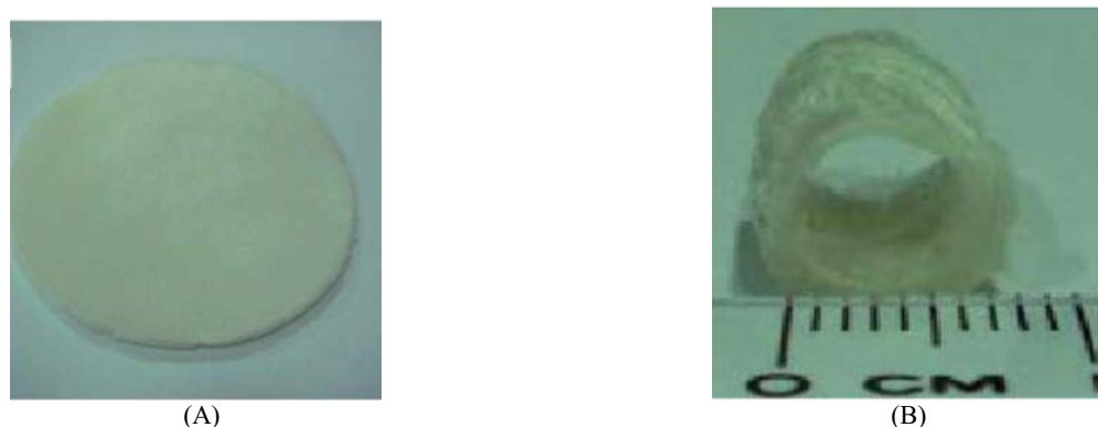
Fig. 1. Morphology of (A) an ionic cross-linked alginate sponge (ICAS) and (B) a new designed nerve conduit (5') with a porous ionic cross-linked alginate/chitosan composite, derived from a crinkled ionic cross-linked alginate sponge (crinkled ICAS) and combined with chitosan (Scheme 2).
