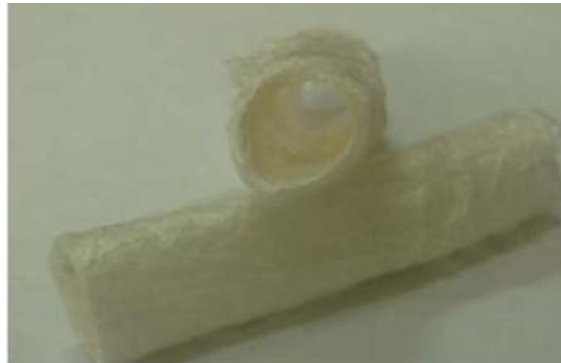
Fig. 3. The morphology of a new designed nerve conduit (7") with a porous ionic cross-linked alginate/chitosan composite derived from a crinkled ionic cross-linked alginate/chitosan sponge (crinkled ICAS) and additional cross-linking reaction with \text{CaCl}_2 (Scheme 2).
