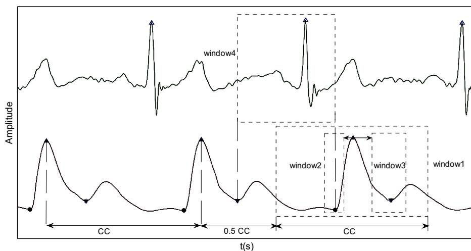
Fig. 1. Windowing methods in feature point extraction.
