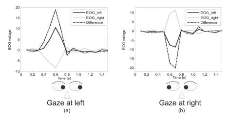
Fig. 3. Gaze direction result from EOG. (a): When subject gazed at left, the left EOG channel (*black line*) is positive while the right one (*dash-dot line*) is negative. Therefore, the difference (*gray line*) between the left and right EOG channel is positive. (b): When subject gazed at right, the voltages of the two EOG channel are inverse and their difference is negative.
