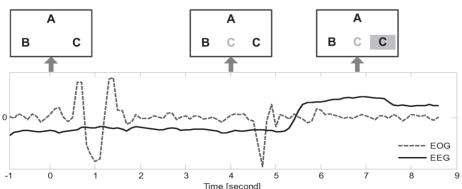
Fig. 4. Detailed process of a target selection task.
