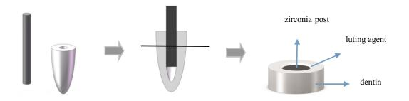
Fig. 1. The schematic illustration of the post cementation.
