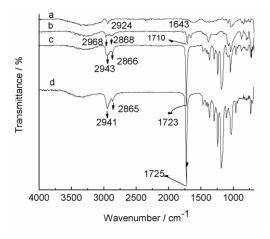
Fig. 2. FT-IR spectra of PHCSO-g-PCL.
