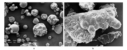
Fig. 3. SEM analysis of (a) CSO and (b) PHCSO-g-PCL (×500).
