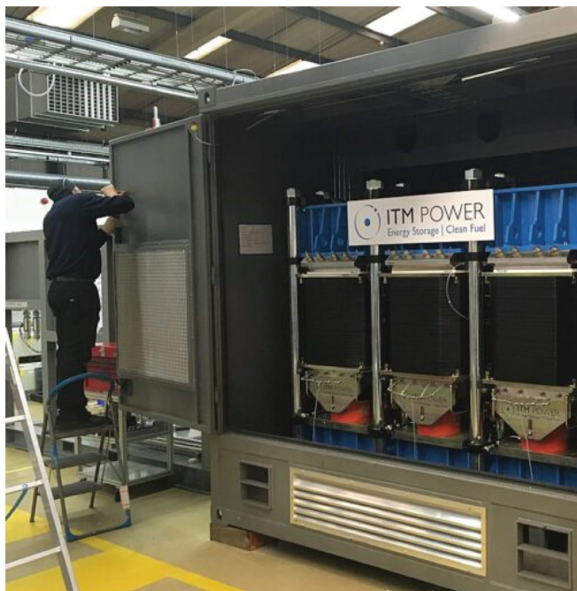
A two-megawatt electrolyser. Representative image. Photo by Bubble60/Wikimedia Commons.
