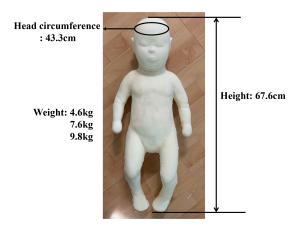
Fig. 2. The specification of the developed infant dummy.
