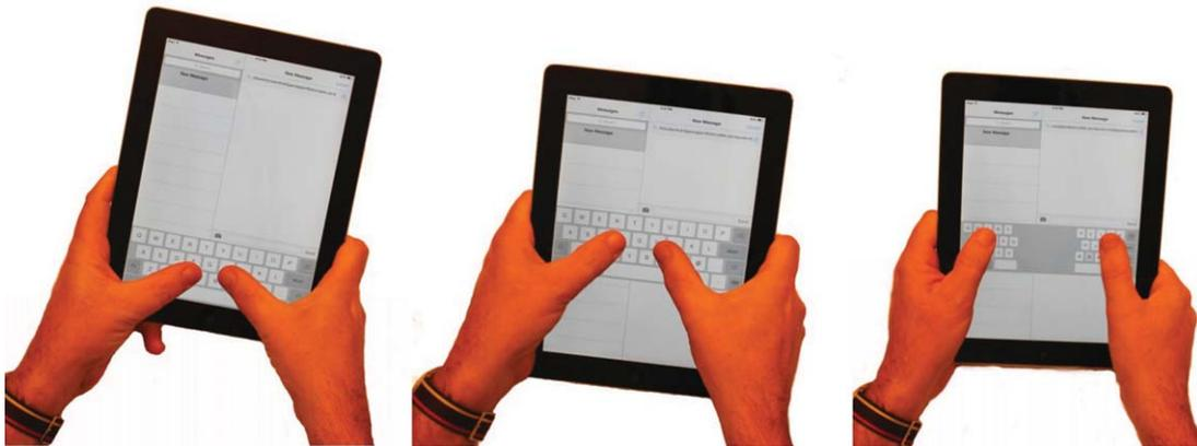
Fig. 5. Using two hands to operate a tablet to type on the keyboard is often associated with wrist extension, wrist ulnar deviation, and extension of the thumb joints. Moving the keyboard up into the middle of the tablet (middle) and using the split keyboard function (right) improves postures and comfort.
