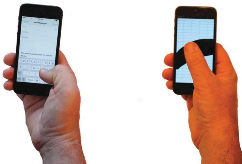
Fig. 4. When icons and buttons are located near the base of the thumb the thumb takes on a non-neutral posture (left photo) whereas when icons and buttons are placed along an arc as noted by the black area in the figure on the right the thumb posture takes on a more neutral posture. The phone on the right is displaying an image of the optimal area for thumb reach as described by Otten et al. [46]
