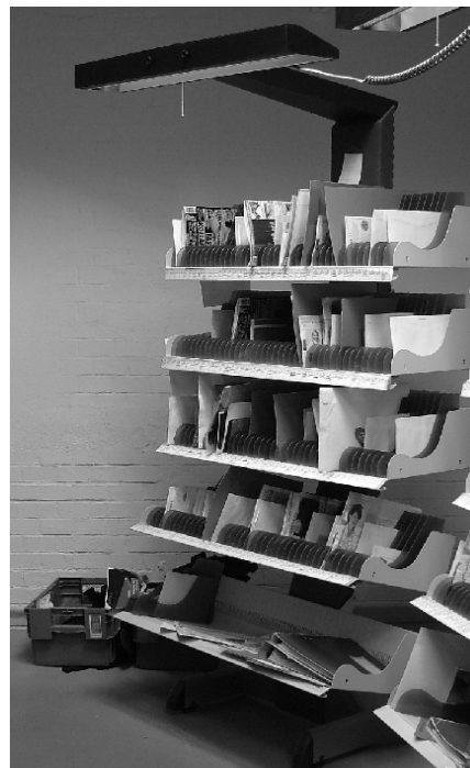
Figure 1. The sorting rack with the new lighting. The top shelf should be at shoulder height for the postal worker.
