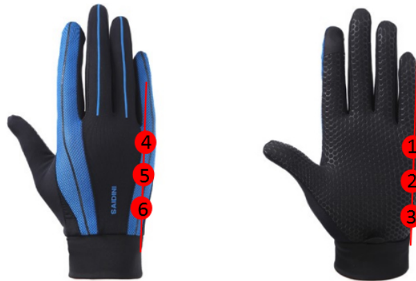
Fig. 1. Inspection points* of Tuina data gloves (*Test points: ① ② ③: side of small thenar side; ④ ⑤ ⑥: dorsal side of thenar).
