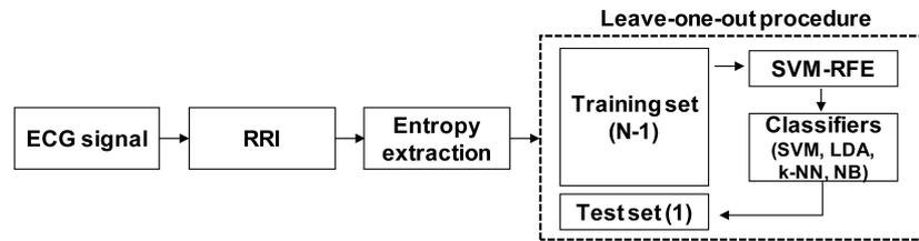
Fig. 2. Overview of data processing procedure.
