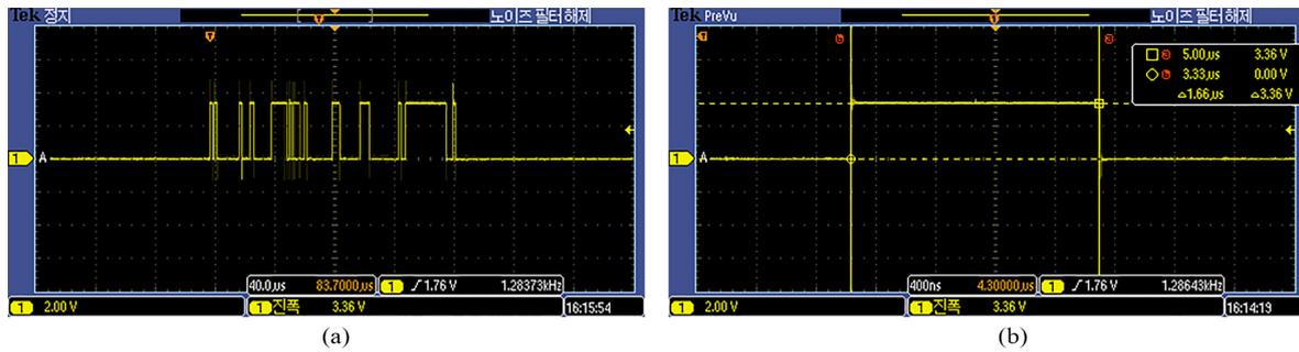
Fig. 9. Working performance of the smartphone dongle communicating wirelessly with the lighting device. (a) One data package is received from the lighting device, (b) data rate.
