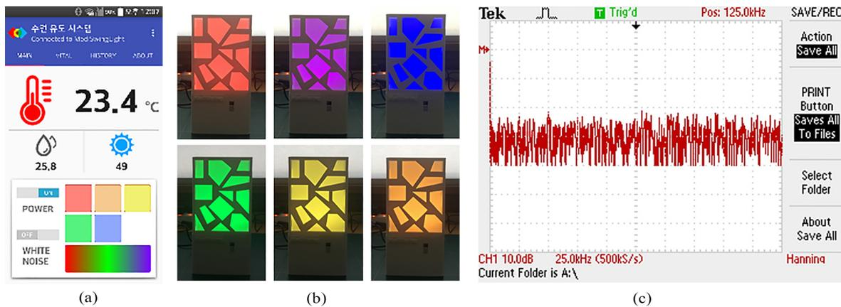
Fig. 10. Use of the smartphone application to control the manufactured lighting device, (a) developed smartphone application based on the Android operating system, (b) Using the smartphone application to control the manufactured sleep-lighting device. (c) White noise output of the lighting device in the frequency domain.
