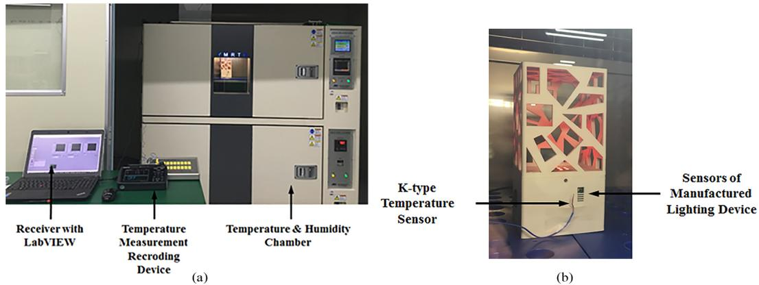
Fig. 5. Experiments for testing the temperature and humidity measurement performance of the proposed lighting device. (a) Image of the assembled sleep-lighting device used in the temperature and humidity measurement performance tests. (b) Using K-type thermocouple sensor to observe the temperature measurement performance of the sleep-lighting device.
