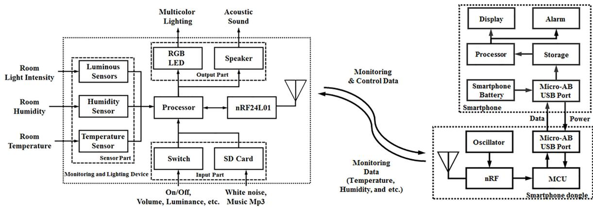
Fig. 2. Diagram of proposed smart sleep-lighting system.
