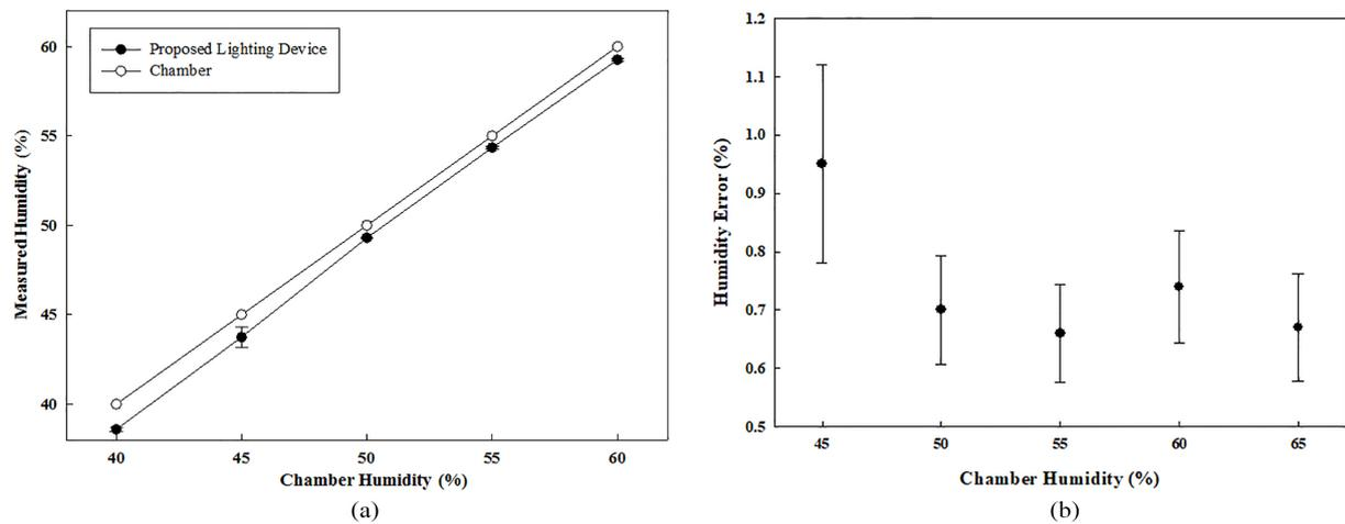
Fig. 8. Comparison of the proposed lighting device with humidity setting value of the chamber, (a) humidity measurement test between the proposed lighting device and the chamber displayed value, (b) error value of the measured humidity value between proposed device and the chamber displayed value.
