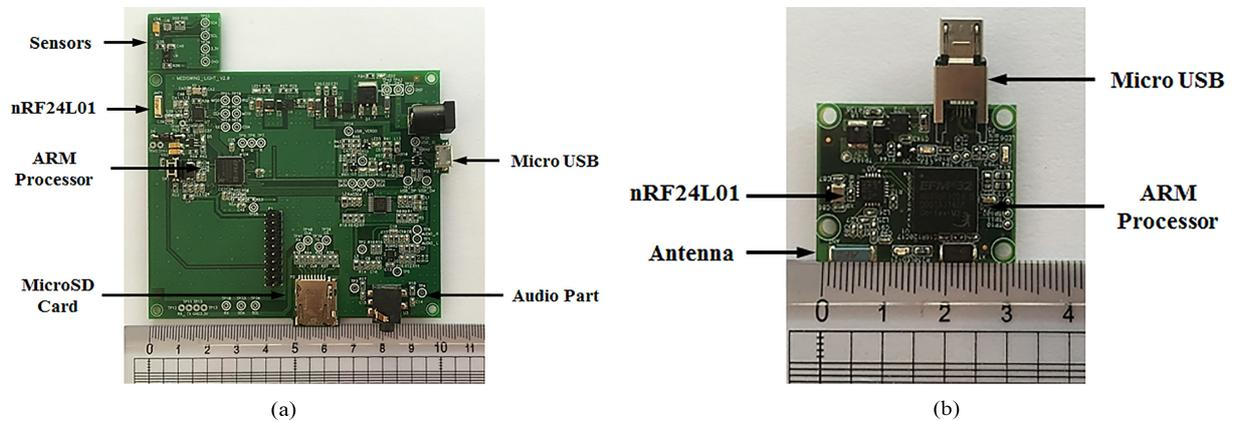
Fig. 4. Pictures of the manufactured smart sleep-lighting system PCBs, (a) Manufactured sleep-lighting device PCB, (b) Manufactured smartphone dongle PCB.
