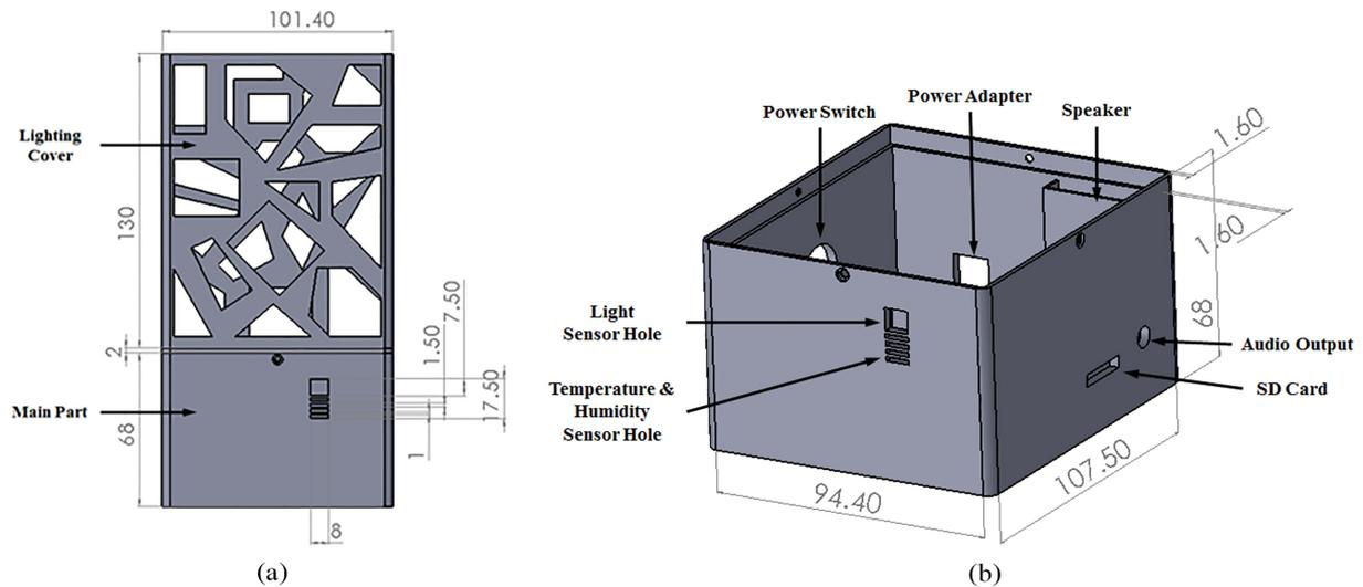
Fig. 3. Schematic of the 3D case model for the sleep-lighting device, (a) external view of 3D sleep-lighting device case model, (b) 3D model for the bottom part of the sleep-lighting device case.
