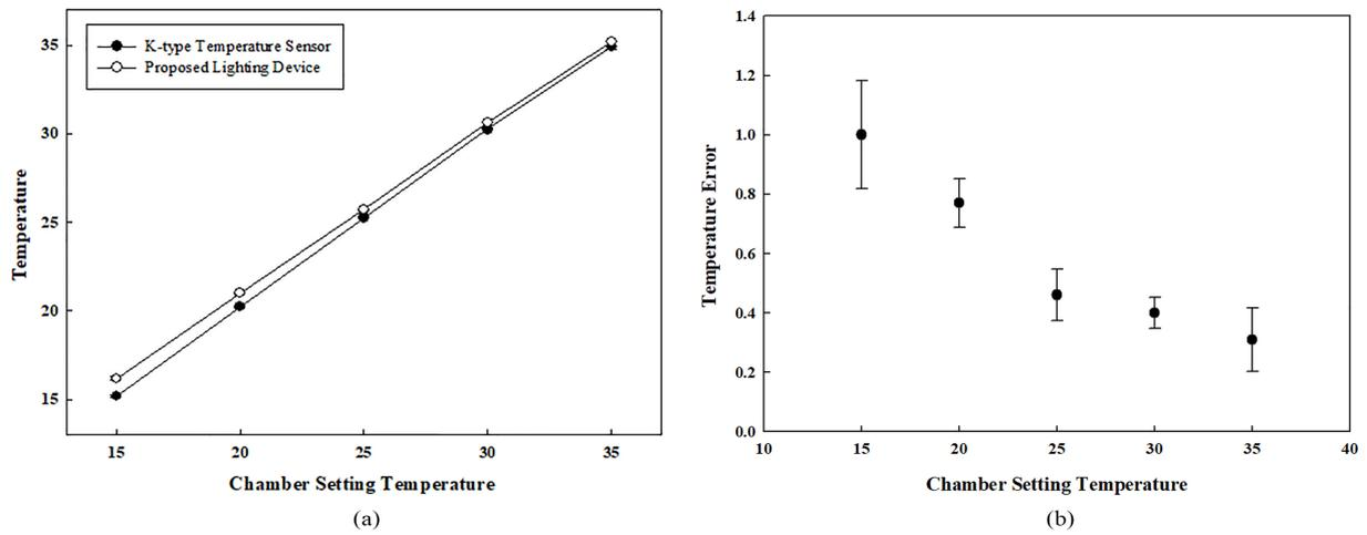
Fig. 7. Comparison of the proposed lighting device with a commercial temperature measurement device in terms of temperature measurement, (a) temperature measurement test between the proposed lighting device and the K-type temperature sensor, (b) error value of the measured temperature value between proposed device and the K-type temperature sensor.
