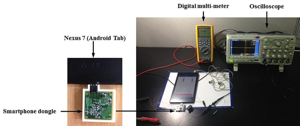
Fig. 6. Wireless communication performance testing of the manufactured smartphone dongle communicating with the sleep-lighting device.
