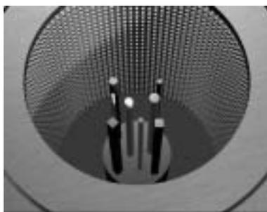
Fig. 1. Fixed arrangement of transducers for 3D ultrasound computer tomography. The transducers are arranged in a cylindrical array around a tank containing the object and water as the coupling medium.
