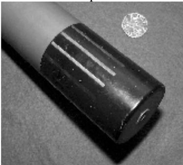
Fig.1: Prototype 16-electrode urethral probe. The diameter is 50 mm. The electrodes are of brass. Contact surface is 2x50mm<sup>2</sup>
