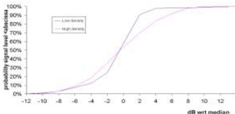
Fig 3: Cumulative distribution function of temporal measurements. Note the adverse effects of *high-density* traffic.
