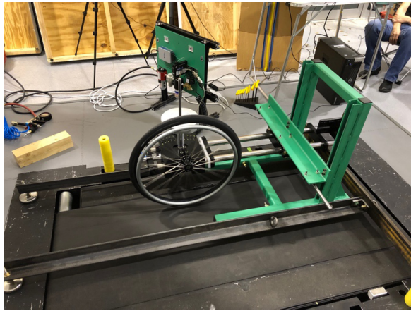
Fig. 8. Treadmill testing with the upper frame and arm assembly.
