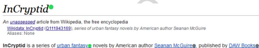
Fig. 2. The Wwyyzerdd user-interface showing linked entities (e.g. genre) in green and unlinked entities (e.g. publisher and author) in gray.
