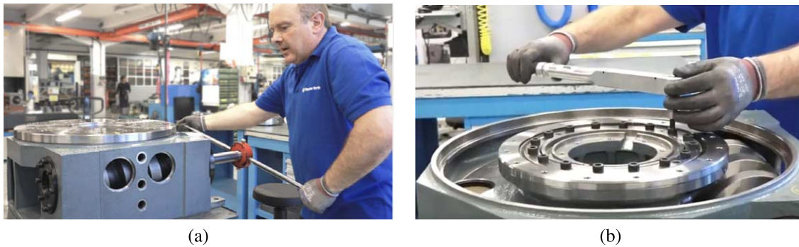
Fig. 8. Working area of the CAPITAL-GOODS scenario (a) and structure of the workpiece (b) where a collaborative robot is deployed to support workers in repetitive screwing/unscrewing tasks.
