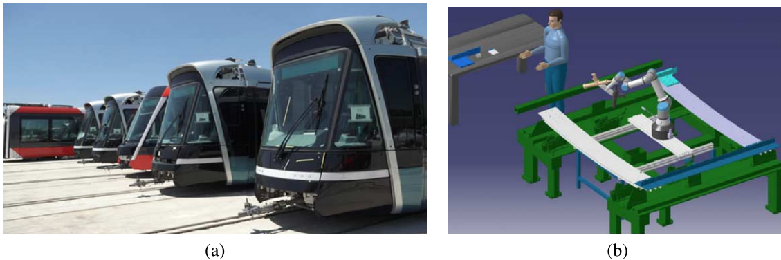
Fig. 9. Design of the collaborative cell of the RAILWAYS scenario to support workers in the assembly of door frames.
