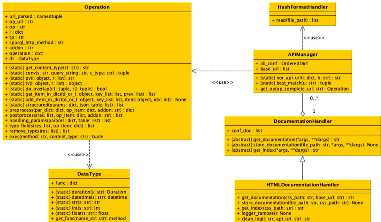
Fig. 3. The UML class diagram of all the Python classes implementing RAMOSE.
