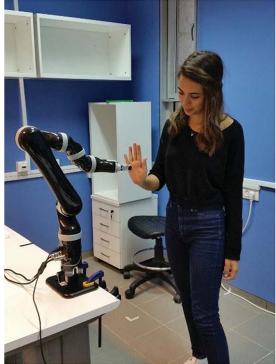
Fig. 4. The experimental setup. Shown here is a participant playing the mirror game with the robotic partner.
