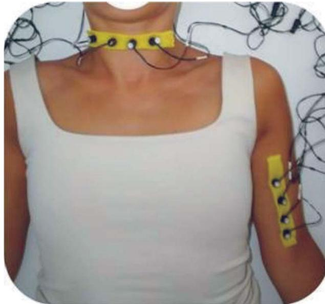
Fig. 2. Solenoid displacement. Subjects judged whether the distance between the active solenoids felt bigger or more intense.
