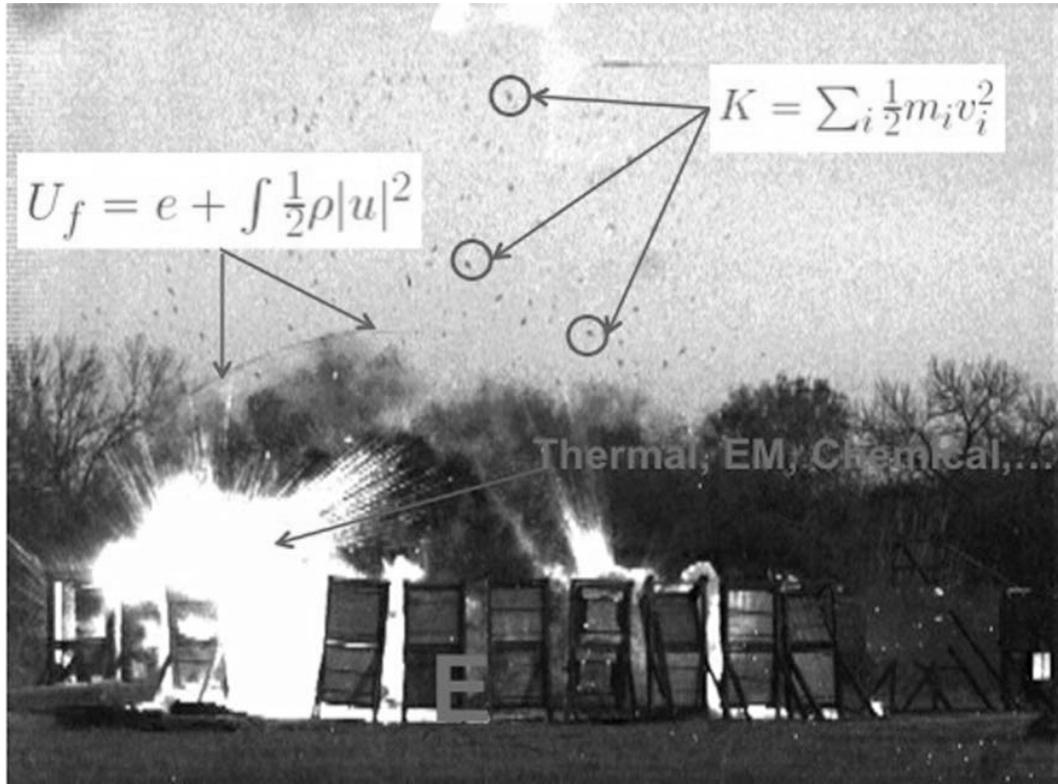
Fig. 1. The total energy conversion from detonation of an explosive charge resulting in kinetic energy of fragments ( $K$ ), and a shock adiabat ( $U_f$ ) together with excess thermal, chemical and electromagnetic pulses (EM). The shock wave and the associated blast wind are responsible for primary blast injury.
