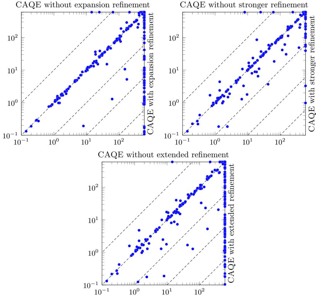
Figure 6: Scatter plot comparing the solving time (in sec.) of CAQE with and without extended refinements (expansion refinement and stronger refinement) and preprocessing using BLOQQER. Both axes have logarithmic scale.
