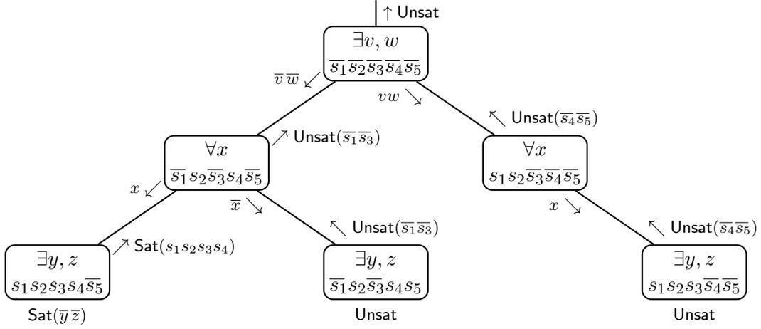
Figure 1: Recursion tree corresponding to the execution of  $\text{SOLVE}_{\mathcal{Q}}$  on the formula  $\exists v, w. \forall x. \exists y, z. (w \vee x \vee y)(v \vee \bar{w})(x \vee \bar{y})(\bar{v} \vee z)(\bar{z} \vee \bar{x})$  as shown in [Example 4](#).
