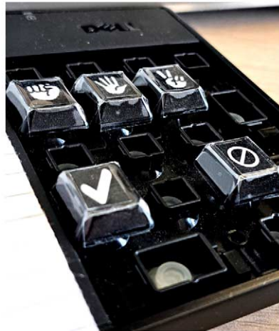
Fig. 5. Tailored control pad used in the second design to interact with the robot.
